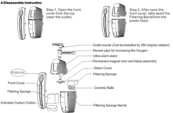
Notice: For some model, there are some small ceramic balls inside, it is easy to spill out when opening the filtering barrel, so we suggest you use a vessel or bag to avoid the ceramic balls Sprinkle all over the floor.
