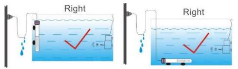
\*Please make the power cable a drip ring shape to avoid the water flow into the socket through the power cable.
